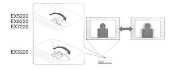
If your image looks like or , you may have placed the projector off to one side of the screen at an angle. Place the projector directly in front of the center of the screen, facing the screen squarely. If you can't move the projector, use the horizontal slider on the projector to correct the image.
