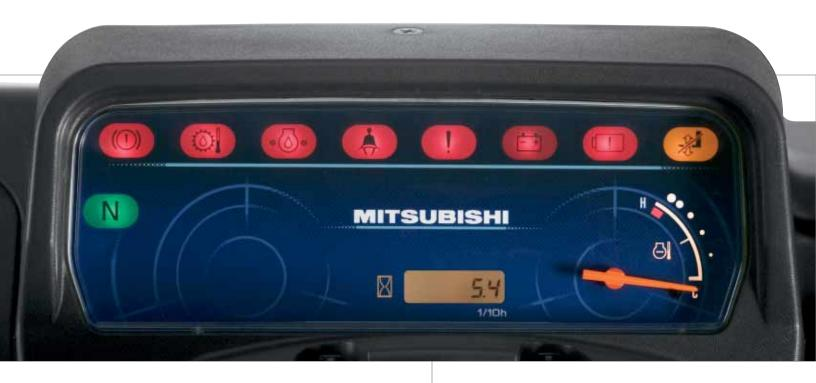
Gasoline and diesel engines include analog fuel gauge.
